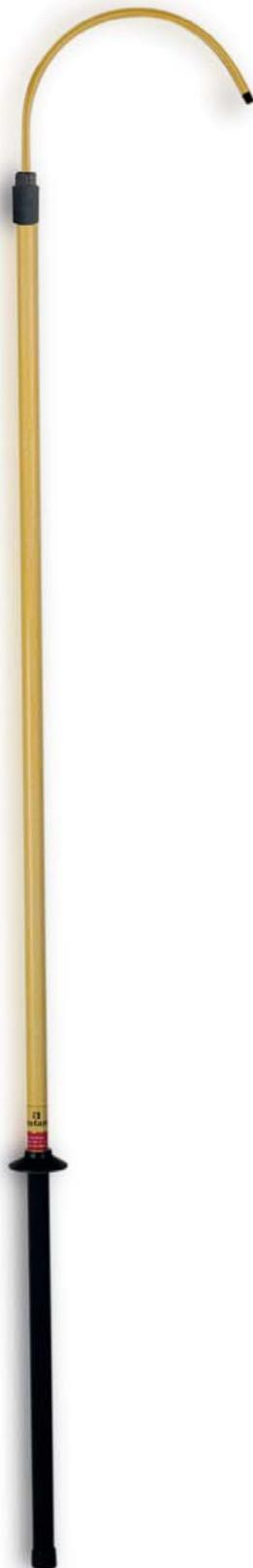
Rescue pole with only one section made of polyester and fibreglass tube Ø 32 mm with humidity-proof seals on each end, hand protector, grip, tip, M-10 metric head and rescue hook.
